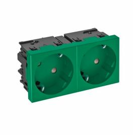
Protective contact socket double 33°, with increased touch protection, with screwless terminals, 2-pin, 16 A, 250 V~, with connection terminals to IEC 60884-1.
